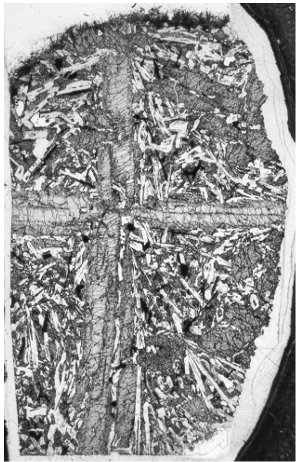
Figure 13: Photomicrograph of thin section 12021,135 illustrating elongate pyroxene crystals growing from a common nucleation point. Section is about 2 cm long. NASA S70-43351.
