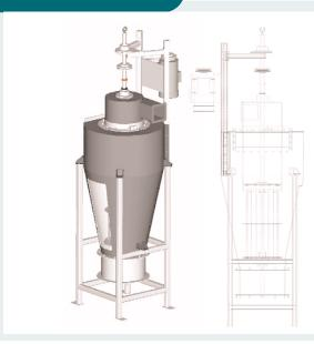
The dynamic cyclone classifier, being developed by InnovaTech, Inc., incorporates a boundrylayer separator within a cyclone housing that allows sharp classification of soft ceramic particles.
