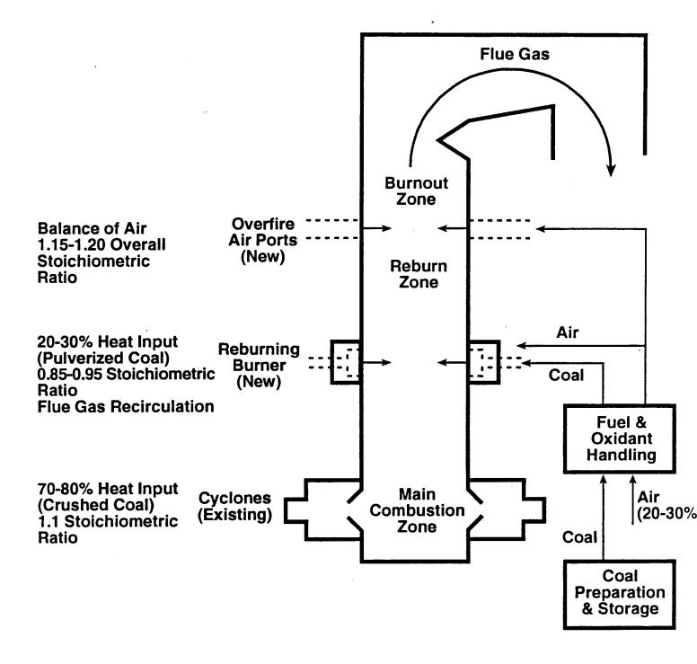
Figure 2. Schematic of Coal Reburning Process
