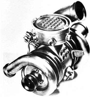
Figure 1.—Brayton Rotating Unit (BRU).
