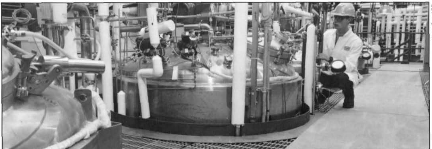
NREL's metabolically engineered Zymomonas biocatalyst will allow cofermentation of both major components of biomass in a single set of tanks, greatly reducing capital equipment and operating costs. These pilot-plant-size tanks are part of NREL's new Process Development Unit.
