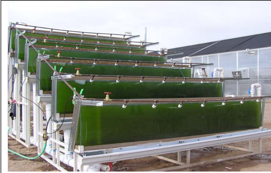
Figure 11. Operation of the multi-stage, continuous-flow photobioreactor for groundwater nitrate removal by Scenedesmus cells.
