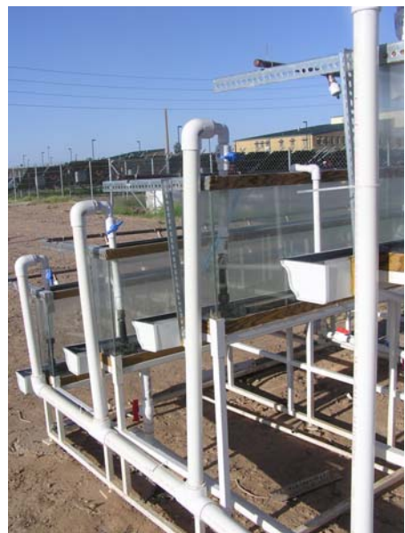
Figure 7. A PVC manifold system conveys compressed air into individual glass tanks for aeration.
