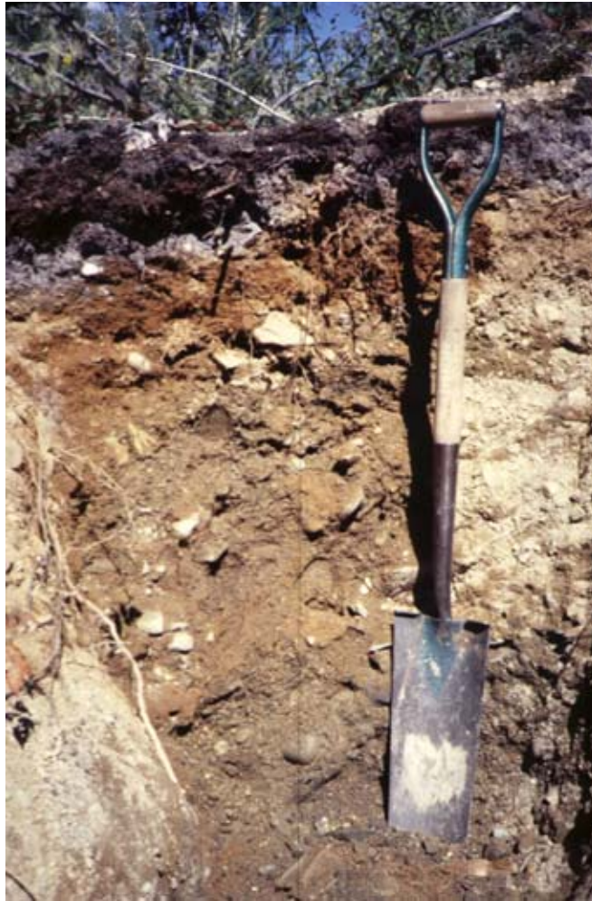
Figure 10.—A soil profile of Hermon sandy loam from a wooded area of Hermon-Monadnock complex, 8 to 15 percent slopes, very bouldery.
