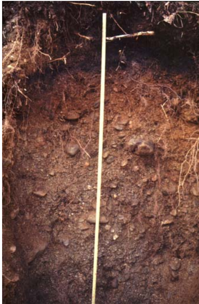
Figure 11.—A profile of the Masardis soil from a unit of Masardis fine sandy loam, 3 to 8 percent slopes.
