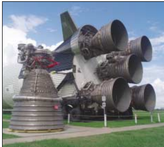
This close-up view features a single F-1 rocket engine (left), the first stage and the five F-1 engines on an actual Apollo Saturn V launch vehicle (partially out of frame), which was originally built to start a crew of astronauts on its way to the Moon. These have been on permanent exhibit since 1977 in Rocket Park.
