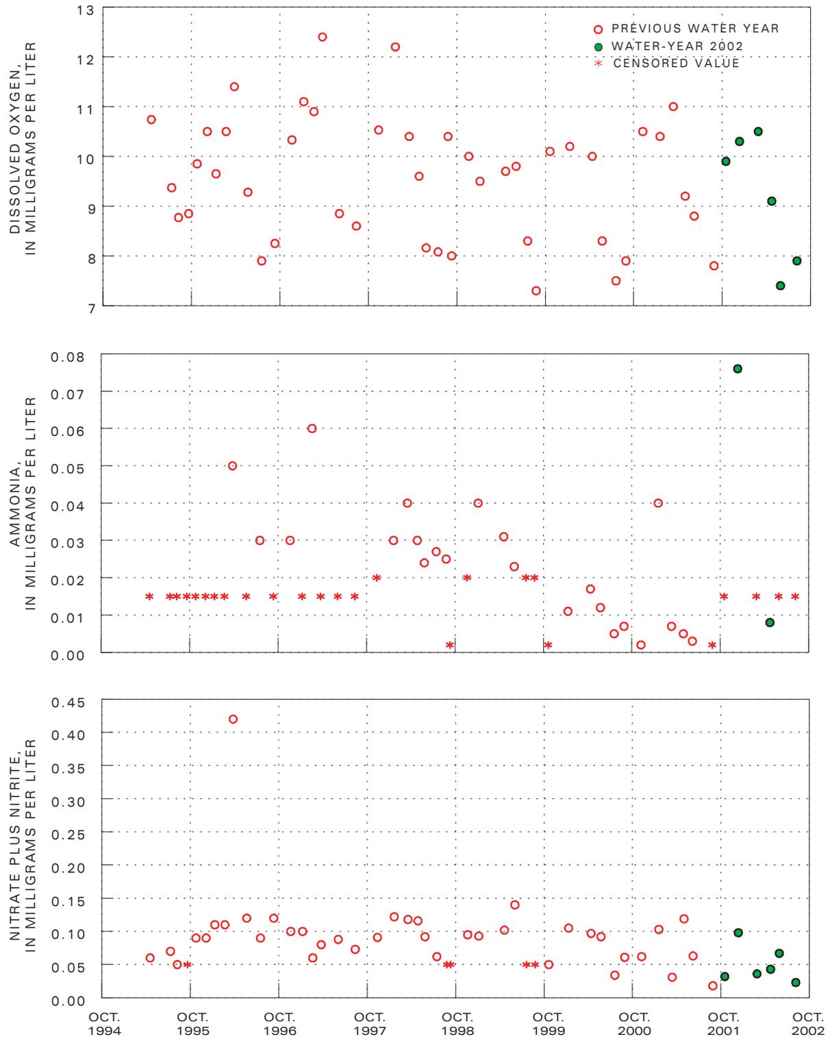
Figure 13. Distribution of selected water-quality constituents relative to time for East River above Slate River near Crested Butte.
