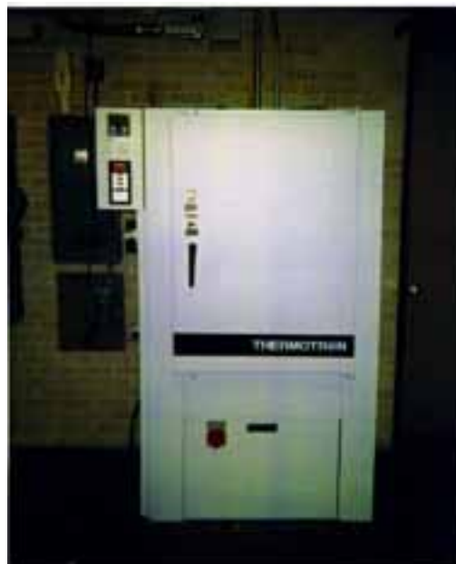
FIGURE 8. THERMOTRON AIR CIRCULATING AGING OVEN USED FOR LONG-TERM ISOTHERMAL EXPOSURE
