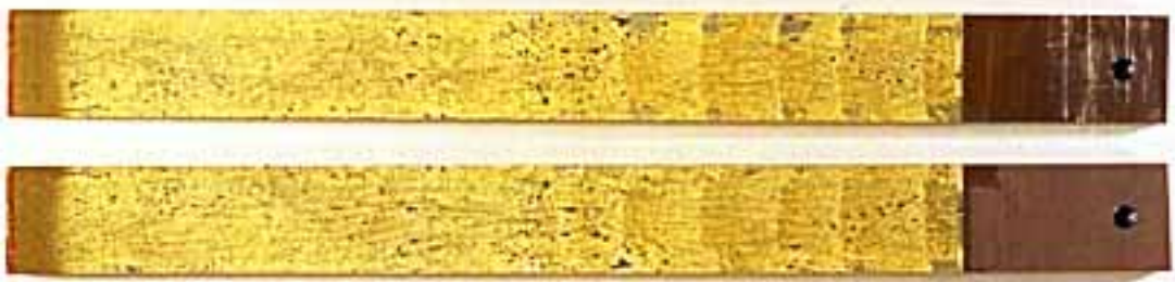
FIGURE 19. FRACTURE SURFACES OF THE Al/FM ® 73M/Al BONDED SYSTEM (AS RECEIVED)
