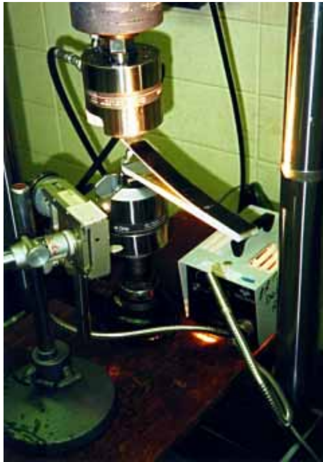
FIGURE 12. DOUBLE CANTILEVER BEAM SPECIMEN BEING LOADED IN A SERVOHYDRAULIC TEST MACHINE
