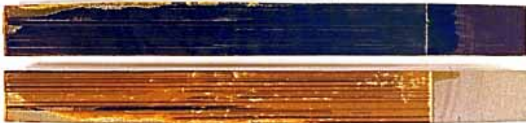
FIGURE 23. FRACTURE SURFACES OF THE Al/FM ® 73M/Al BONDED SYSTEM (AS RECEIVED)
