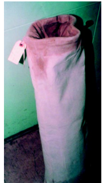
Figure 6-7 and 6-8. Bag filters showing discoloration associated with bypass.
