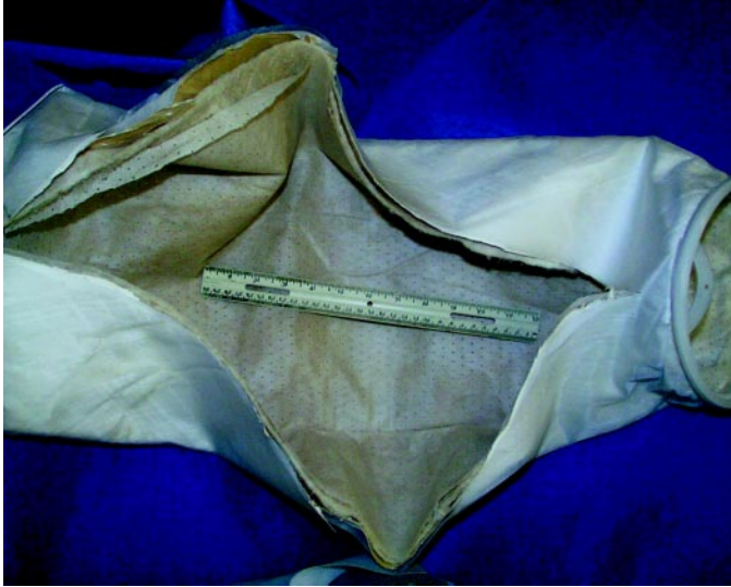
Figure 6-4. Cut-away of bag filter.
