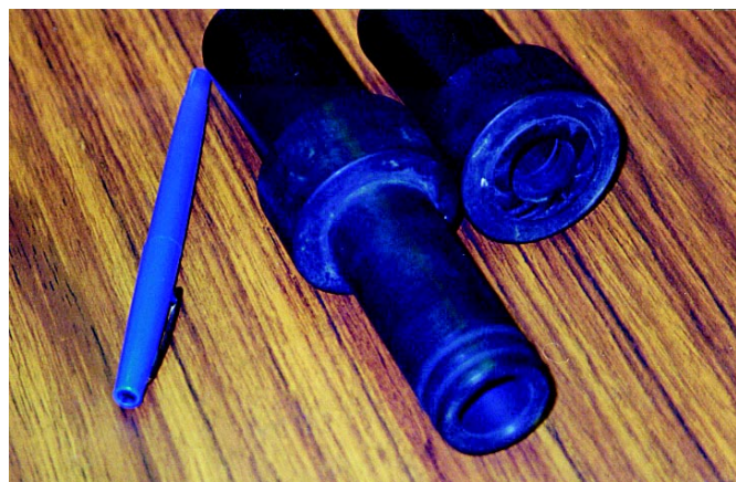
Figure 6-18. Cracked plastic adaptor used between membranes.
