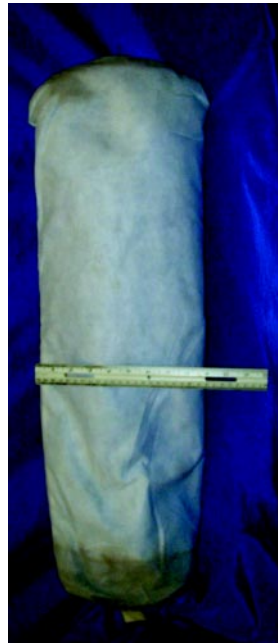
Figure 6-7 and 6-8. Bag filters showing discoloration associated with bypass.
