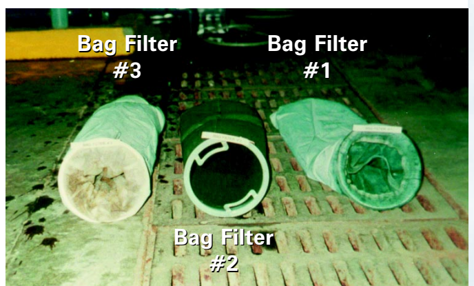
Figure 6-9. Different configurations of bag filters tested. (see Table 6-3)
