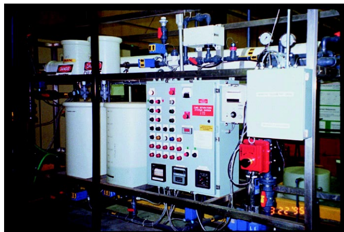
Figure 9-3. Packaged UF System.
