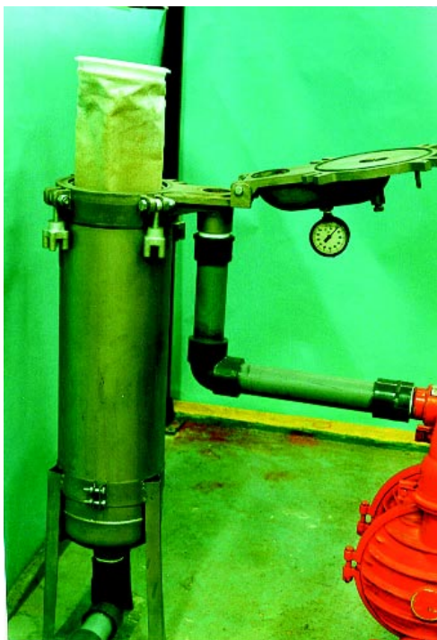
Figure 6-3. Typical bag filter.
