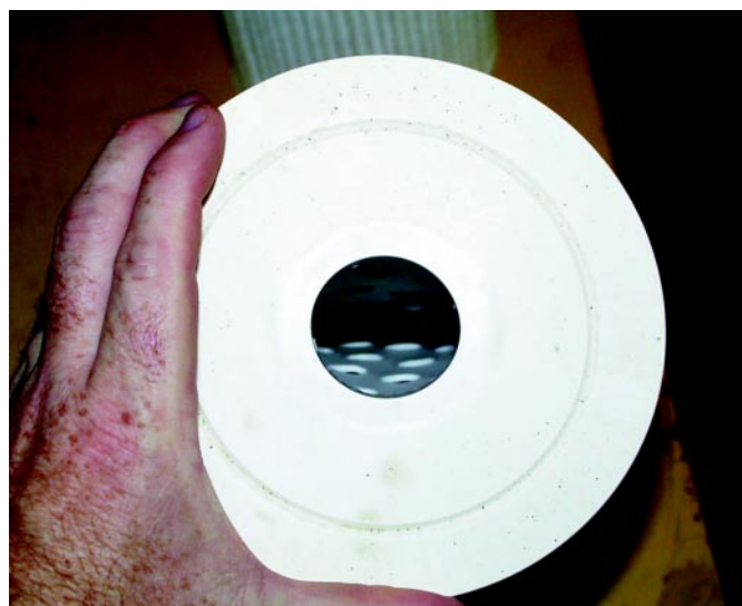
Figure 6-16. Collapsed cartridge filter.
