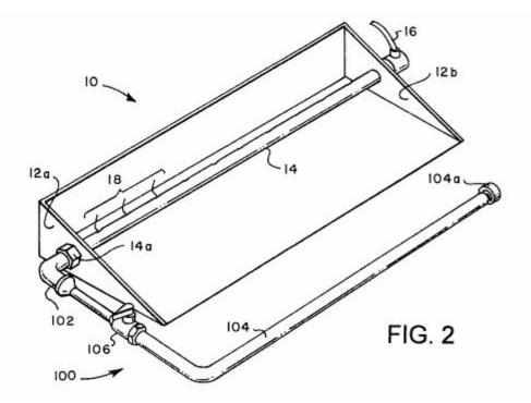
In <u>Golden Blount I</u>, we concluded that the "raised level" limitation in claim 1 refers to the top of the primary burner tube and requires that the top of the primary tube be above the top of the secondary burner tube. 365 F.3d at 1059-60. Likewise, we concluded that the "below" limitation in claim 17 required that the top of the secondary burner tube be below the top of the primary burner tube. Id.
