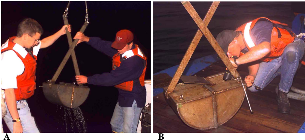
Figure 5. A) Grab sampler being recovered. B) Grab sampler being subsampled.
