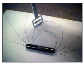
The picture above shows the correct orientation of the Magnaprobe and a few sample lines. This Magnaprobe has a square frame; less expensive models have an oval frame. Demonstrate the correct orientation for your class. The edge of the large oval makes a good straight edge to draw the short line.
