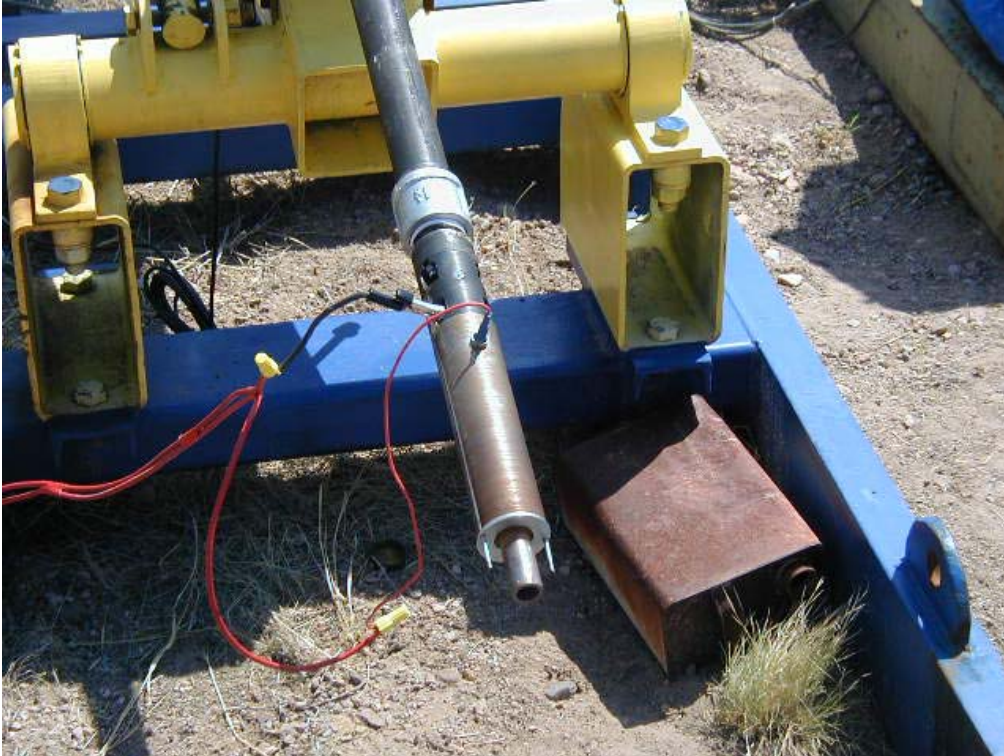
Figure 14. Field burner assembly on drill frame rig with spark plug energized with temporary connection to ignition circuit.
