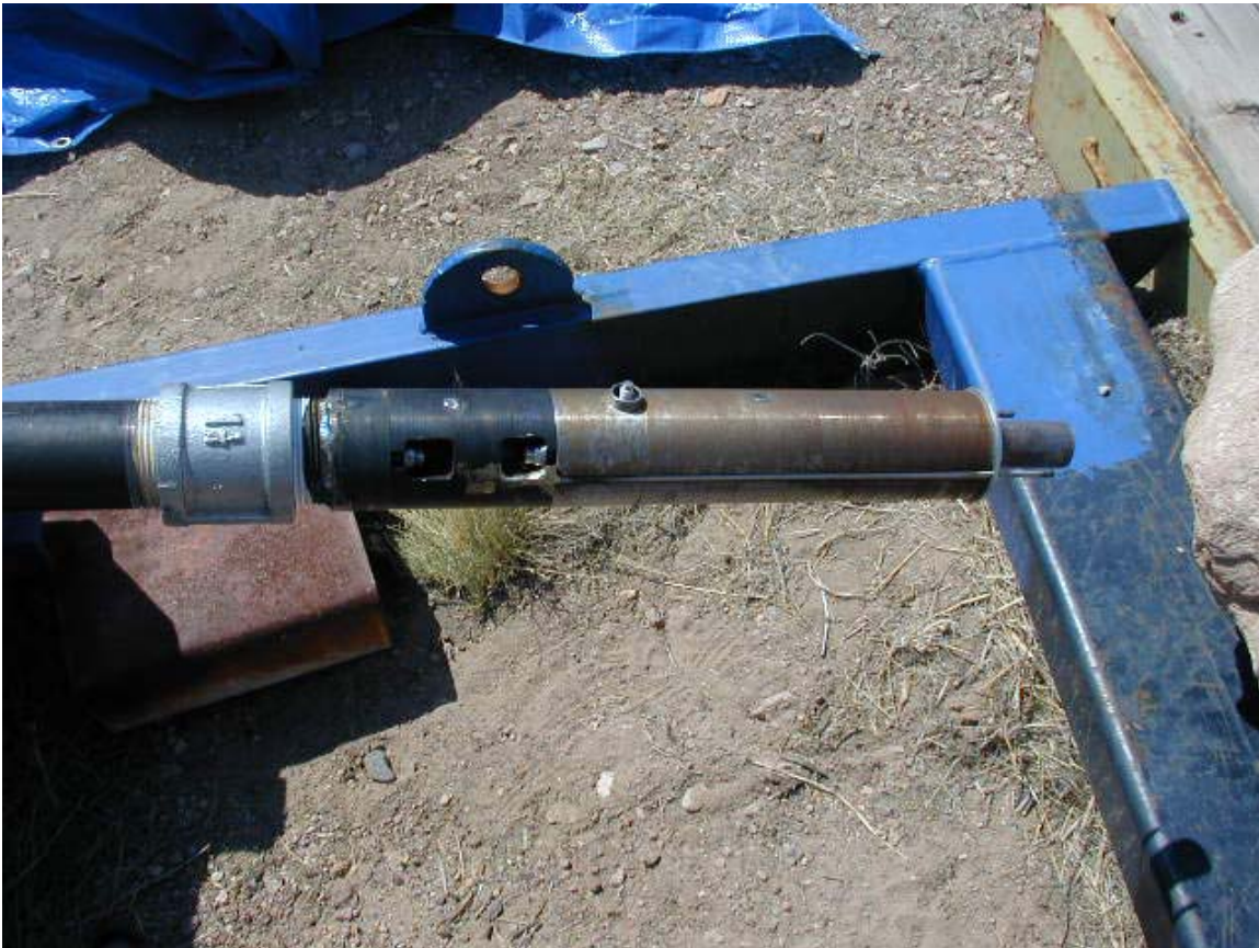
Figure 13. Field burner assembly on drill frame rig with (from left to right) the drill stem, coupling, a cross-over and mixing section, an ignition and gas expansion piece, a flame holder and combustion chamber, an exhaust nipple with internal nozzle (not visible). Cooling water lines are visible on the outside of the burner chamber and exhaust nipple.
