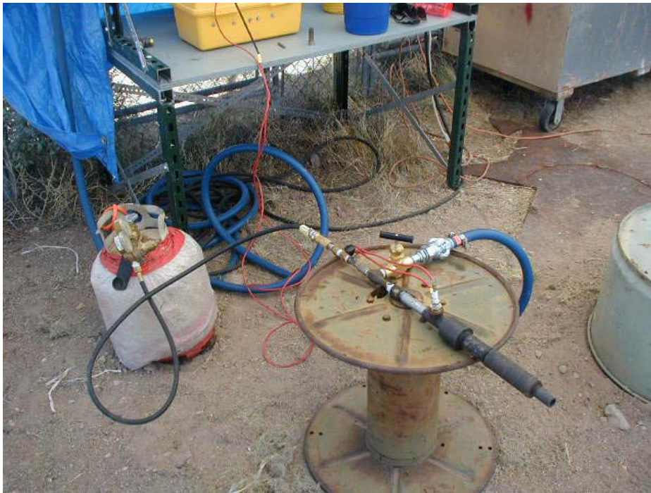
Figure 9. New Mexico Tech bench burner assembly.
