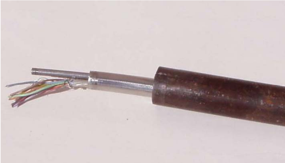
Figure 20. Sample of coiled-tubing fabrication. 1-inch OD coiled-tubing transports the air flow and contains the 1/2-inch stainless tube that transports the coiling water and contains both the telemetry cable and the 3/16-inch OD stainless steel tube that transports the fuel.
