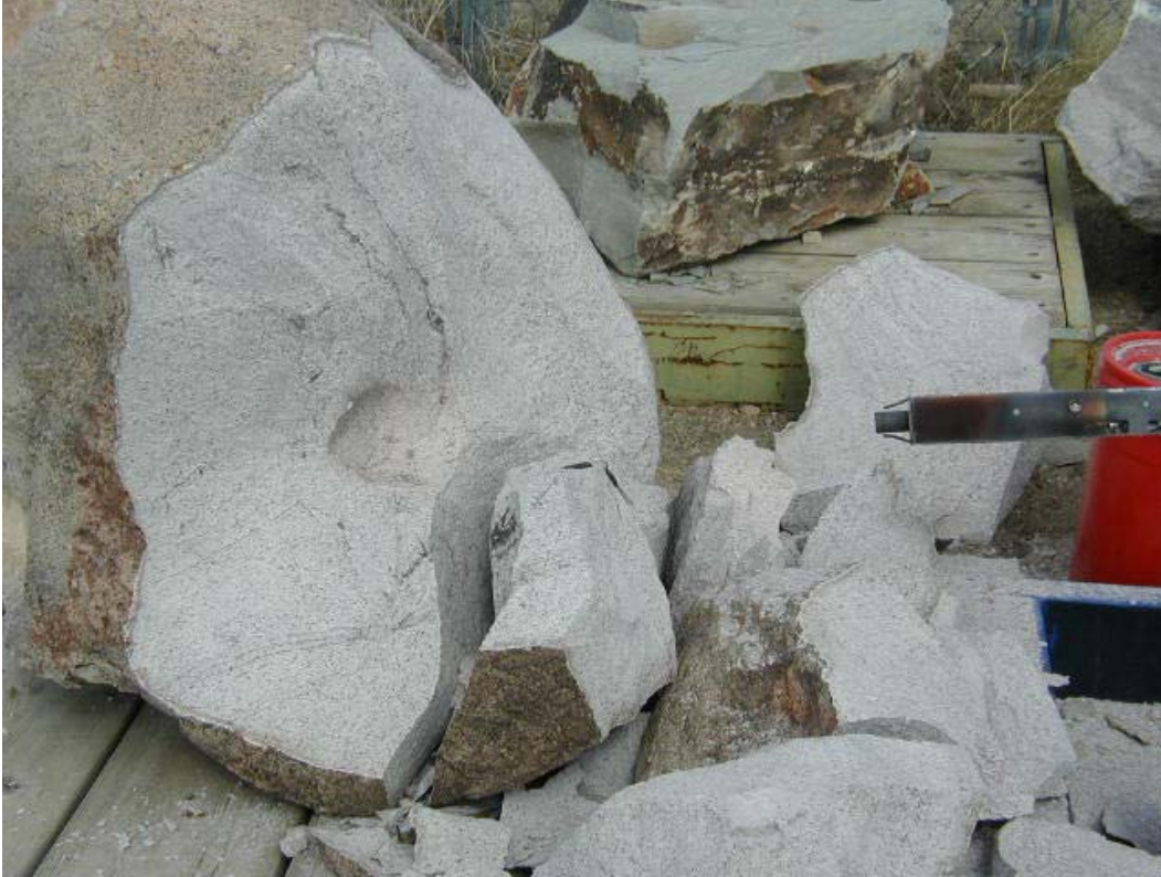
Figure 19. Spallation test on rhyolite sample ended when sample broke into small pieces.
