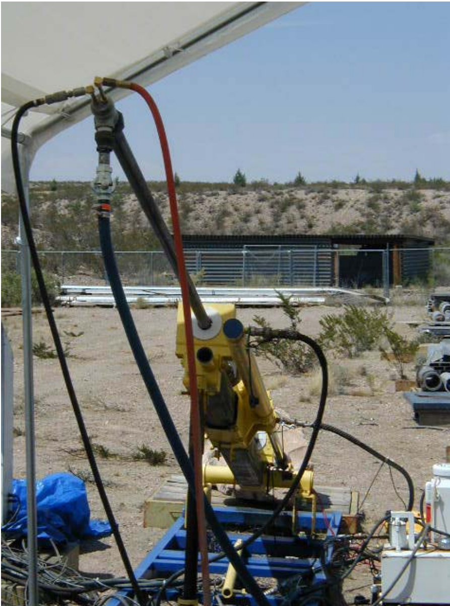
Figure 12. Boart Longyear drill frame with a hydraulic drive system.
