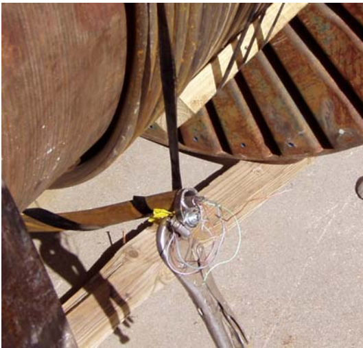
Figure 23. Spark plug testing using the coiled tubing reel to conduct power from the auto ignition to the spark plug.
