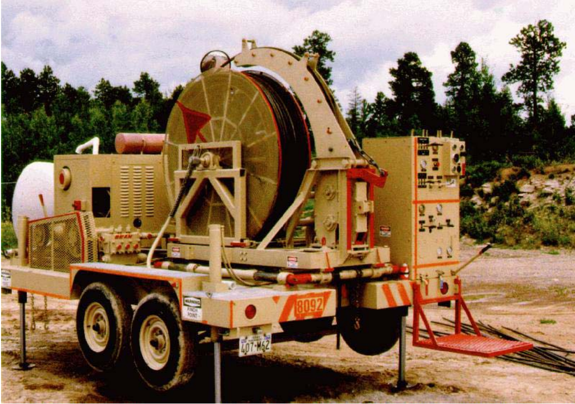
Figure 6. Los Alamos coiled tubing unit configured to support conventional microdrilling.
