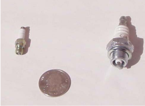
Figure 22. Spark plugs used in tests. The LTD ME-8™ sparkplug is on the left and Champion CJ-8™ is on the right.
