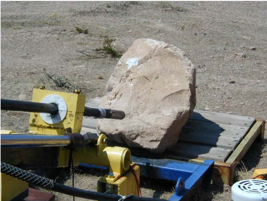
Figure 18. Preparing to conduct spallation test on rhyolite sample.
