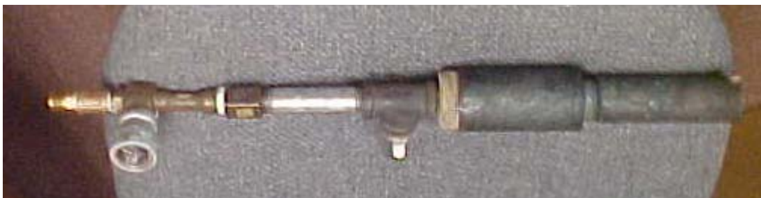
Figure 11. Bench burner assembly with (left to right) propane hose coupling, flow tee for air inlet, mixing venturi, mixing nipple, tee for spark plug mount, burner chamber, and nozzle nipple holder with internal nozzle (not visible) .
