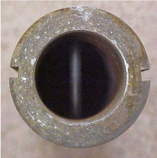
Figure 16. Field burner combustion chamber looking in from bottom. The flame holder is the vertical bar inside the chamber. Slots on the outside protect the cooling water tubings that transport the water from the top of the burner to the nozzle on the bottom of the burner.
