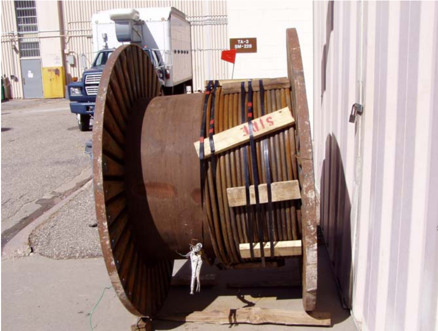
Figure 21. Coiled tubing on storage reel. A 200-ft long coiled tubing procured to demonstrate spallation drilling on Los Alamos coiled tubing unit.
