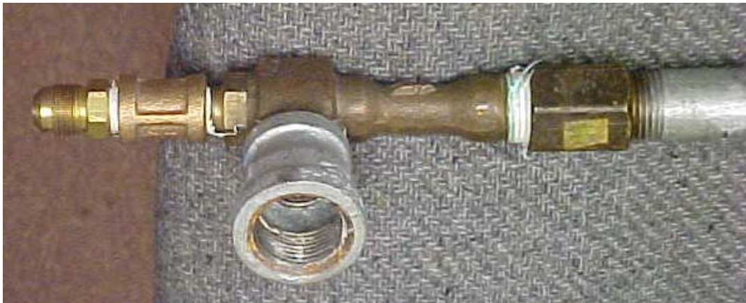
Figure 10. Air-fuel mixing section for bench burner with (left to right) propane hose connector, coupling, flow tee with air inlet on side, venturi, coupling, and mixing pipe nipple.
