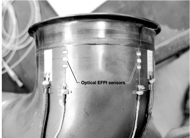
Figure 2. Example of 10 th stage duct instrumentation illustrating the optical EFPI strain sensor.
