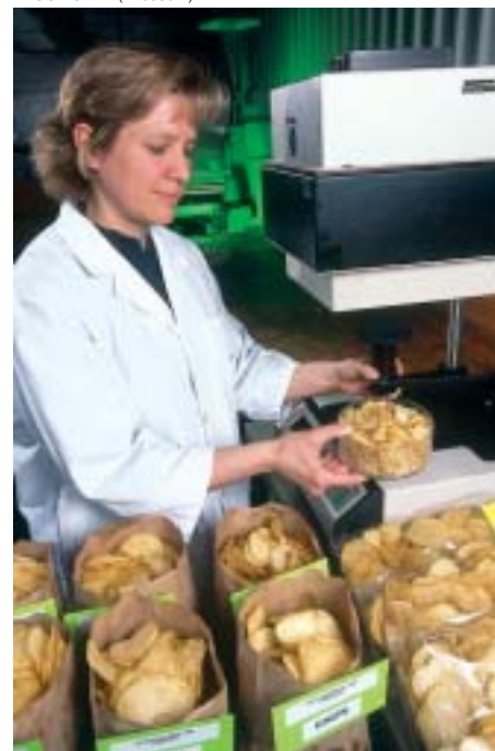
Technician Rebecca Lindlauf measures potato chip color in different breeding lines submitted for evaluation.
