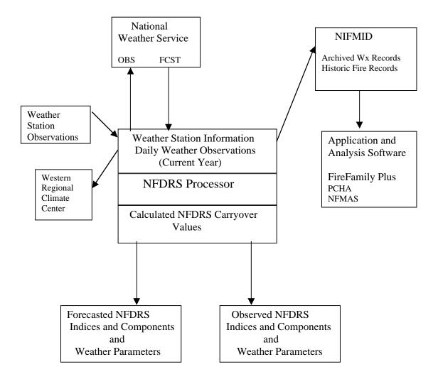
2.0.2 Figure 2 - Flow of Information In and Around the NFDRS Processor
