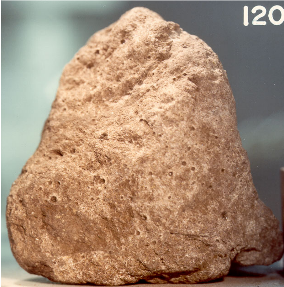
Figure 1: Photo of exterior surface of 12010,12 showing patina and micrometeorite craters. NASA S84-39792. Sample is about 2 x 3 inches.
