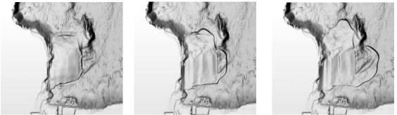
Snapshots from a numerical simulation of the 1964 Seward waterfront slide. The three images show the position of the underwater slide at 10, 30 and 50 seconds after the slide was triggered by strong ground shaking due to the  $M_w$ =9.2 earthquake.
