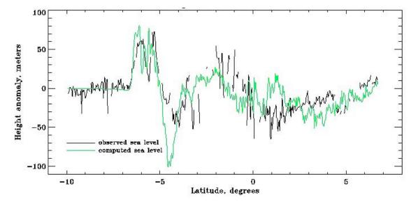
Comparison between observed and calculated sea level heights along the Jason track 129. Sea level heights were calculated from the shallow water equations of motion and continuity. Three source functions of the December 26, 2004 North Sumatra earthquake were constructed and tested against observation data.
