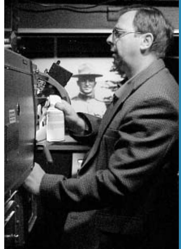
Ed Autry, an audiovisual technician at the Harry S. Truman Library in Independence, MO, uses compressed air to clear debris from the film gate of a 35mm projector. (Photo by Jamie Oakes)
