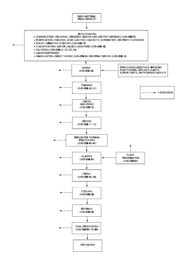
Figure 11.7-1. Process flow diagram for ceramic products manufacturing. (Source Classification Codes in parentheses.)
