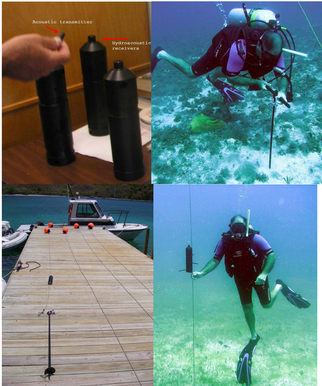
Figure 5. Acoustic transmitters, hydroacoustic receivers, and mooring design and deployment.
