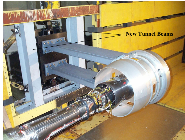
Fig. 12. Wind Tunnel Modifications for RAN Installation
