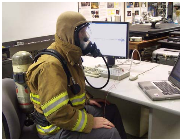
Figure 3. Photo showing data collection station and SCBA equipment.
