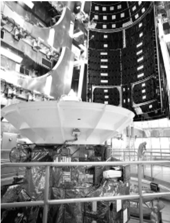
LARGEST interplanetary spacecraft ever launched — More than half of the Cassini/Huygens mass of 12,295 pounds is liquid fuel, required for braking into orbit around Saturn. Here, the payload fairing is hoisted in place around the spacecraft at Launch Complex 40. Cassini's high-gain antenna — the light conical structure — is the upper most element of the spacecraft.
