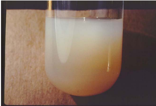
Fig. 3. Nano-diamonds precipitate as a cloudy white gel from acidic solution but they completely “dissolve” in basic solution. Photo courtesy of Roy S. Lewis.
