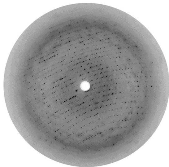
Figure 2 Diffraction pattern of yeast ADH crystals at beamline 17-ID at the Advanced Photon Source.
