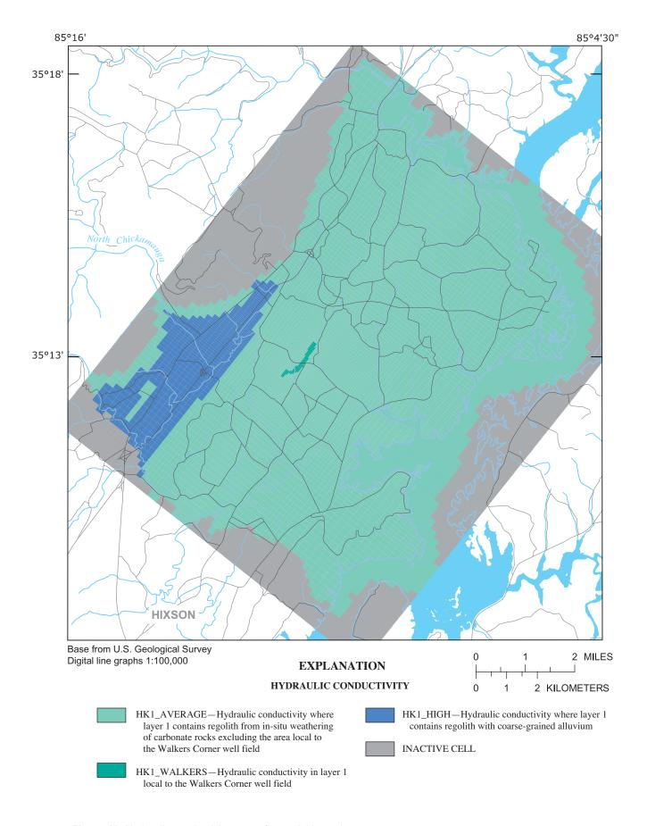
Figure 18. Hydraulic-conductivity zones for model layer 1.
