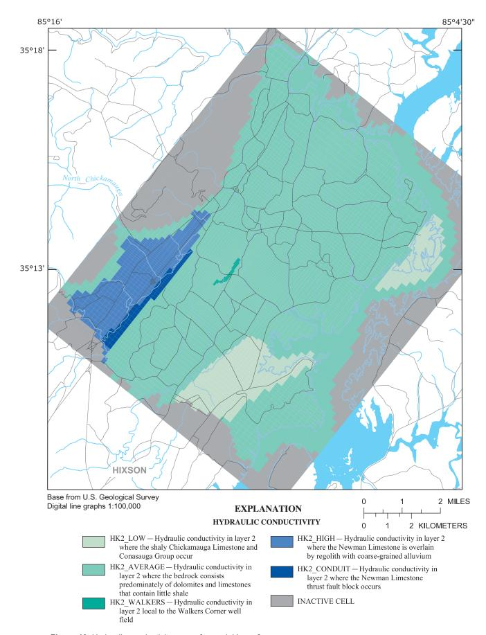
Figure 19. Hydraulic-conductivity zones for model layer 2.
