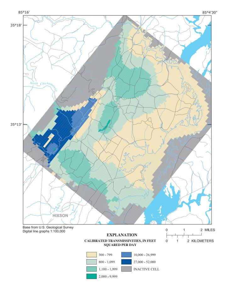
Figure 21. Calibrated transmissivities for model layer 1.
