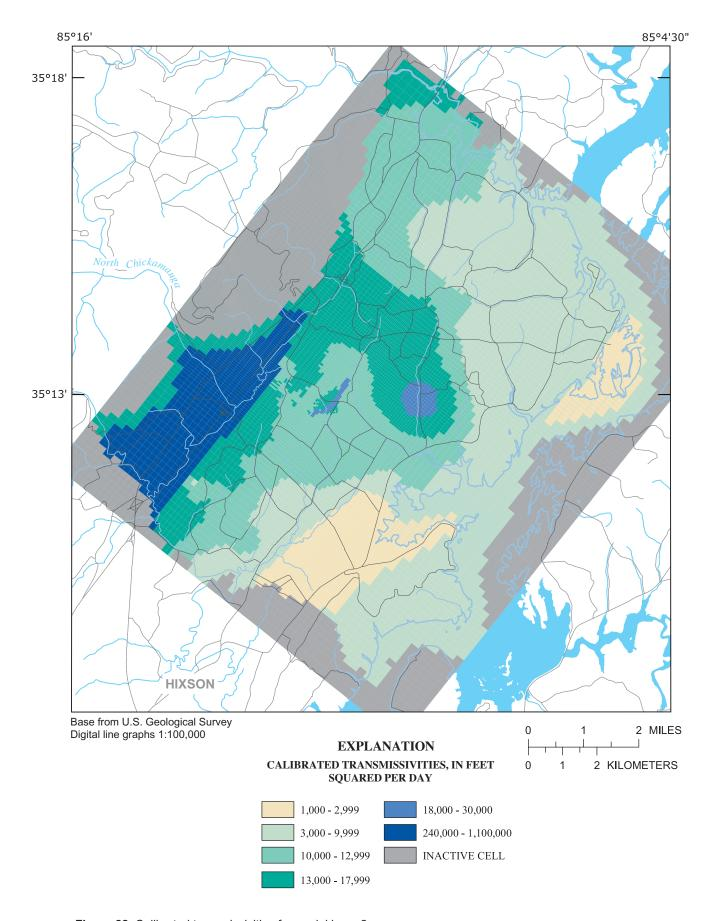
Figure 22. Calibrated transmissivities for model layer 2.
