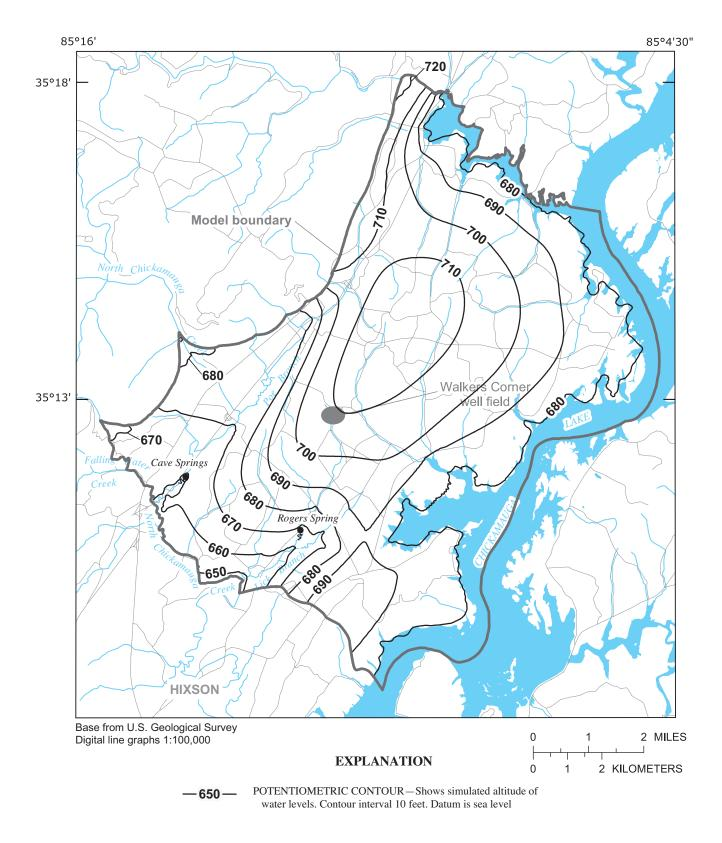
Figure 20. Model-simulated steady-state water levels with no pumping at Walkers Corner well field, layer 1.
