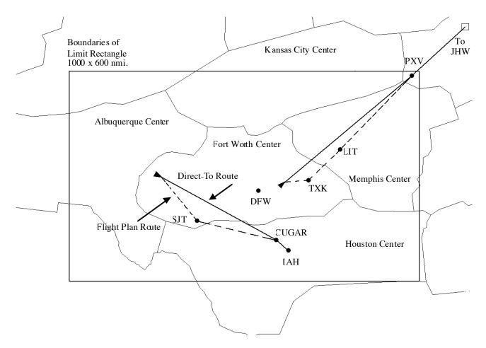
Figure 2. Limit rectangle superimposed on Fort Worth Center airspace. Also shown are two examples of direct-to routes.
