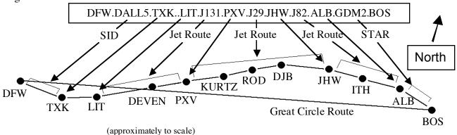
Figure 1. Decomposition of a flight plan into its waypoints and horizontal route segments. For reference, great circle route between DFW and BOS is also shown.
