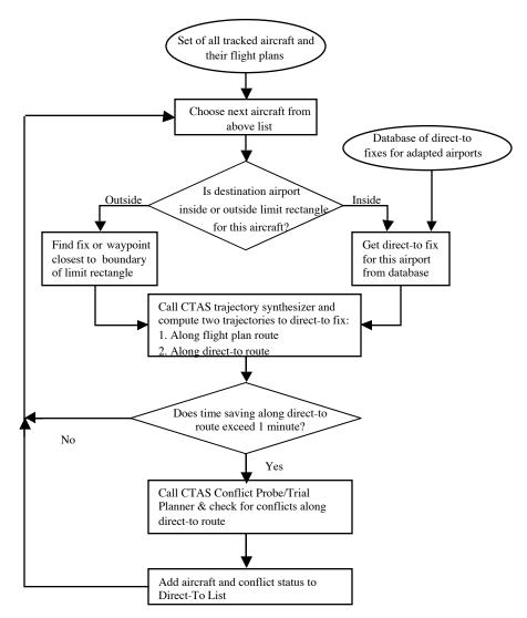
Figure 3. Flow chart of direct-to algorithm.
