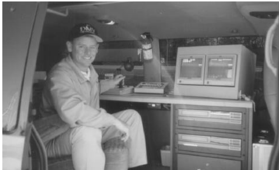
Figure A-2. The IRISystem minivan interior with video screens, VCRs and the joystick which operates the camera.
