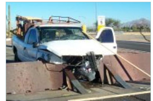
Figure 3-3. Pop-up barrier stops vehicle
