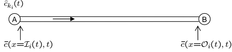
Figure 1: Link Boundary Designation. \mathcal{I}_i(t) indicates the inlet of the link, based on the current flow direction, while \mathcal{O}_i(t) indicates the outlet of the link. The index k_i(t) always refers to the node connected at the inlet.
