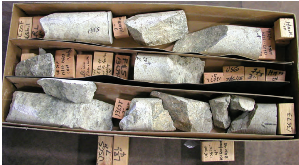
A. Subsurface core collected from bottom interval of exploratory hole UE-20f; deepest hole drilled at Nevada Test Site. Core sample shows welded volcanic tuff from 13,670- to 13,686-foot interval. Wooden blocks indicate sections of core removed from U.S. Geological Survey Core Library. Photograph taken by Jerry Magner, U.S. Geological Survey.
