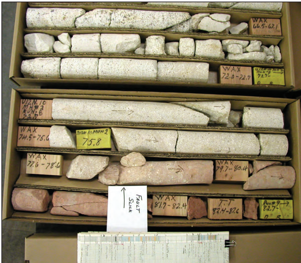
Figure 10. Example of subsurface fracture characteristics in vertical core hole MH-2 in floor of emplacement drift U-12n.10 at 303.77 feet from portal opening, Nye County, Nevada. Core sample shows slickensides and black staining on fracture surfaces at 79 feet. Photograph taken by Jerry Magner, U.S. Geological Survey.
