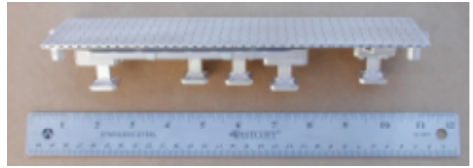
Figure 7: Final brazed 10x40 subarray shown in feed network test configuration.
