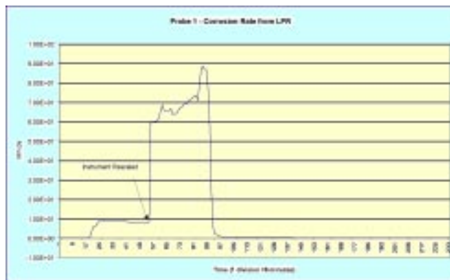
Figure 6. Electrochemical response from reducing gas composition
