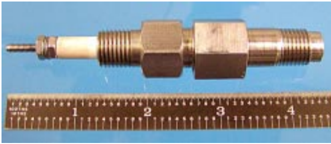
Figure 8. Configuration of an electrochemical probe for firewall insertion
