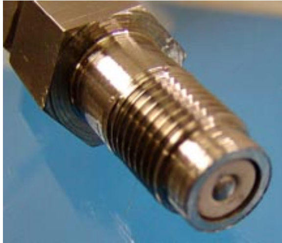
Figure 9. Configuration of an electrochemical probe for firewall insertion
