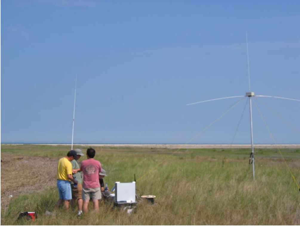
Figure 5. Long range HF Radar Receive Antenna (located to right of picture) located on Cedar Island, Virginia during field testing activities held in June 2005.
