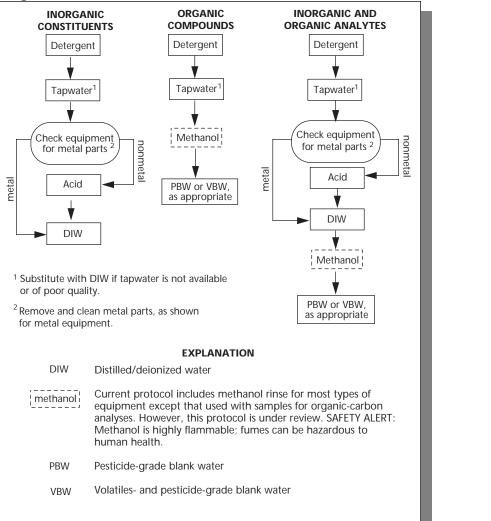
**Figure 3-1.** General sequence for cleaning equipment before sampling for inorganic and (or) organic analytes.
