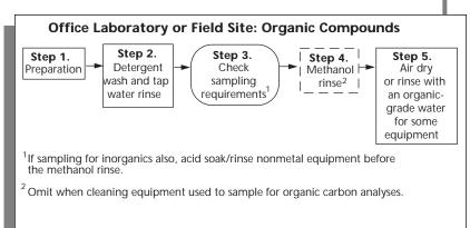
**Figure 3-4**. Cleaning procedures for equipment used to sample for organic compounds.
