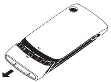
3 Remove the battery cover by following the instructions in "Removable Battery" step 2. Lift the battery cover to remove it.
