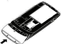
**5** Replace the battery cover by following the instructions in "Removable Battery" step 5.
