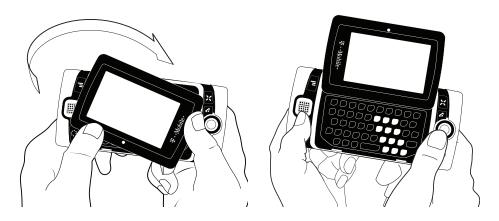
Alternatively, use your right index finger to push down gently on the upperright corner of the display. The screen will spring into the open position.
