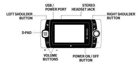
**DIRECTIONAL PAD (D-Pad)** – Press up, down, left, or right to scroll or move within text fields, and navigate in the browser or games. By default, the D-Pad navigates folders and screens, jumping over individual items. You can make the D-Pad navigate the same as the trackball (moving item-by-item) from the **Jump Menu > Settings > Trackball & D-Pad** settings screen.
