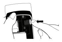
I Forcing the memory card out before pushing to release it may cause the card or slot to break.
