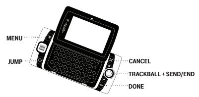
TRACKBALL - Press the trackball to select a highlighted item or press and hold to open a pop-up menu. Roll the trackball to reverse or advance the current selection through the "selectable" items on a screen. Rolling the trackball left or right with a folder highlighted opens/collapses folder contents. Adjust trackball speed and acceleration from the Jump Menu > Settings > Trackball & D-Pad screen. Read what the trackball colors mean during sleep in "Trackball light indicators" on page 34.
