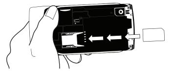
**4** To remove the SIM card, use your finger to press down gently and slide the card right. When it's free of the bracket, lift the card to remove it.
