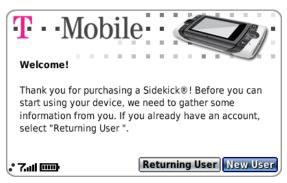
Press the trackball to select the **New User** button and advance to the next screen. On subsequent screens, select the **Next** button to advance.
