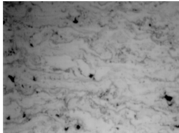
33μm Figure 10: HVOF copper deposit
