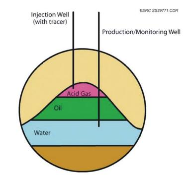
Figure 2. Illustration of top-down injection and production scheme
