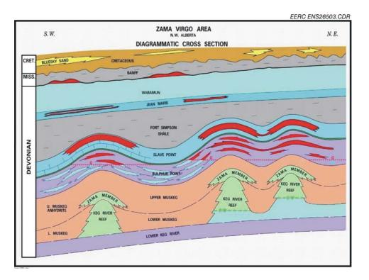
Figure 6. Schematic cross section illustrating the sedimentary succession in northwestern Alberta. Also shown are oil and gas occurrences.
