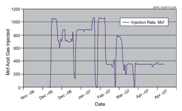
Figure 10. Current acid gas injection profile for the Zama Keg River F pool.
