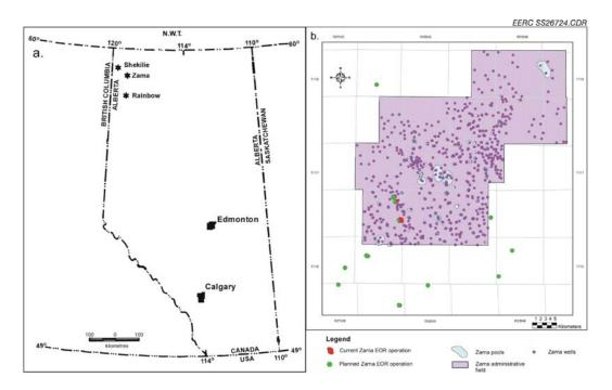
Figure 4. Location of the acid gas EOR project at Zama: a) Keg River hydrocarbon fields in northern Alberta (Apache Canada Ltd., 2003) and b) the Apache Canada Ltd. Zama-Keg River acid gas EOR sites in the Zama oil field. Well locations shown are those where the Keg River Formation was penetrated.
