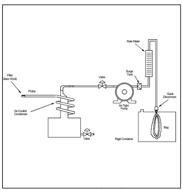
Figure 3-2. Integrated Gas-Sampling Train.
