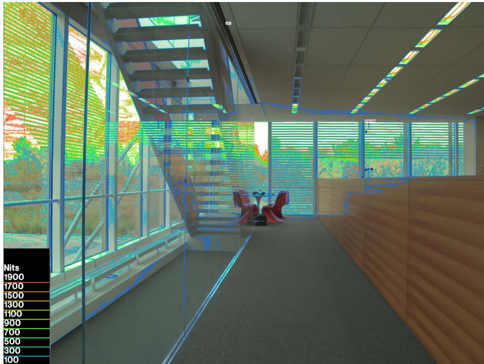
Fig. 3 Iso-contour analysis generated from a HDR photograph capturing the staircase area on the south part of the mockup. (Multiple exposure images are taken on 10/25/2004 between 16:04:36 – 16:05:23; aperture size of f/4; shutter speed between 1/4 - 1/500 sec; partly cloudy sky)
