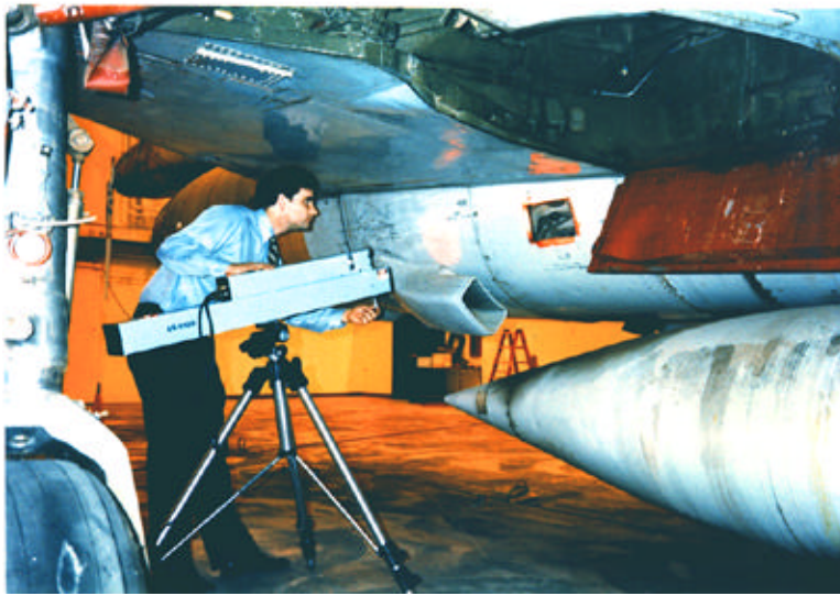
Figure 11a: Tripod mounted shearography camera/laser is shown inspecting an aircraft (Laser Technology, Inc.).
