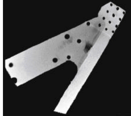
Figure 6: Reverse Geometry image of corrosion on a horizontal stabilizer of an F-111 aircraft (Digiray).
