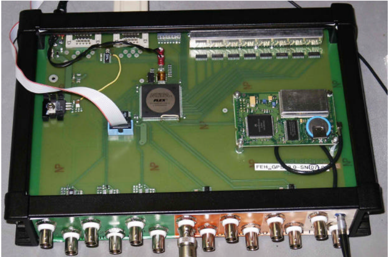
Figure 40: Photo of the GPS module at the test bench: The front panel holds the BNC connectors for input and output signals; the status LEDs, the LAN connectors, the RS232 interface and the “Reset” push button are on the back side. Also visible are the Motorola receiver (right) and the FPGA (center).
