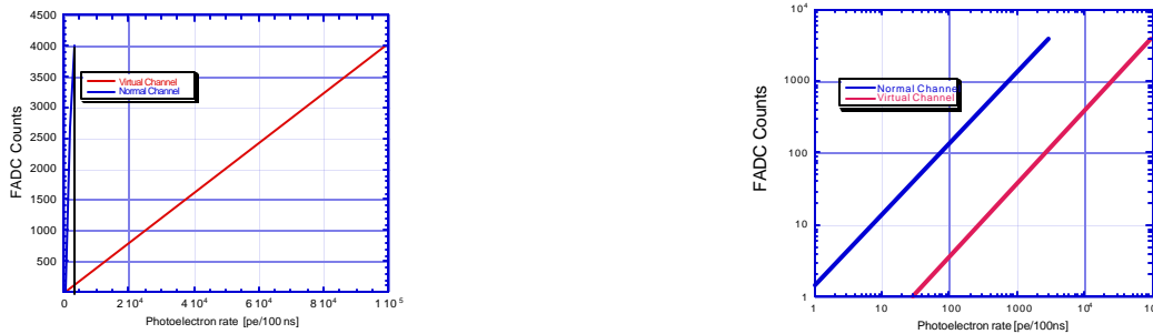
Fig15: The normal (blue) and virtual (red) channel transfer characteristics in linear and logarithmic scales.
