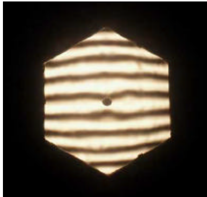
Figure 1.8 Ronchi test of a glass mirror surface. Parallelism of the fringes shows the regular spherical surface of the mirror. Irregularity in the shape would be seen as irregularity of the fringes.
