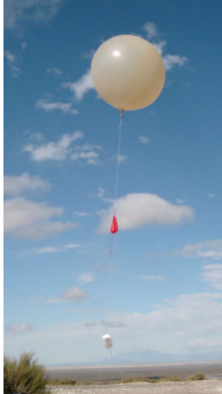
Figure 1: Radiosonde launched with helium filled balloon.
