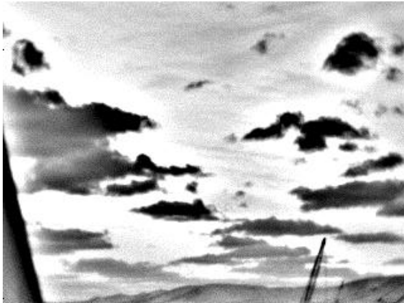
Figure 1.24 A cloud image taken with a Raytheon Series 2000B camera from the top of the physics building in Adelaide - looking north-east. Its a pyroelectric 320 \times 240 pixel camera sensitive to 7-14\mu\text{m} infra-red radiation. A negative image is shown - dark (cloud) areas are warm compared to white (clear sky) areas. The image shows cumulus cloud low over the Adelaide Hills - at least 10 km distant. Some closer cumulus is evident in the middle of the image. This foreground cumulus is in front of some higher altitude diffuse/cirrus type cloud (faintly visible in the upper centre of the image). On the left is part of the physics building and in the lower right a construction crane. The horizon is the Adelaide Hills.
