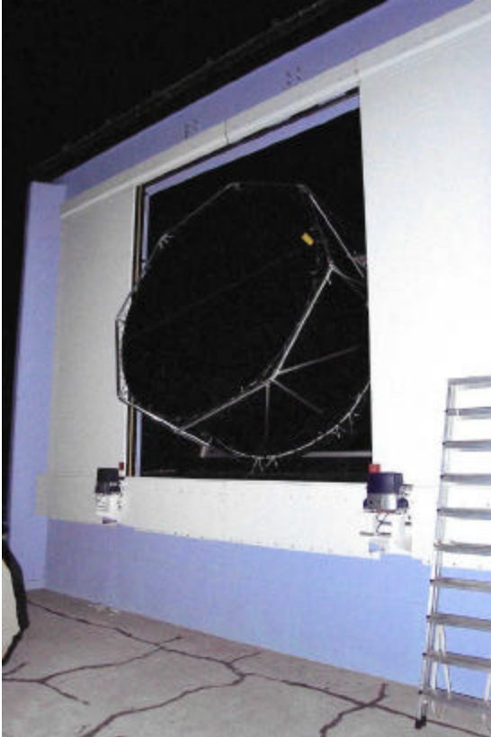
Figure 1.22 Drum calibration device mounted on the outside of the building at Los Leones.
