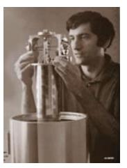
undergoes a rapid change in electrical resistance when heated by the absorption of a single X-ray. The instrument uses a NIST-developed mini-refrigerator that cools the detector chip to an operating temperature near absolute zero (0.1 K). Such cold temperatures are necessary to achieve high resolution, especially for lower energies.
