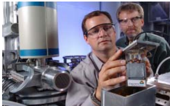
At Argonne's Advanced Photon Source, researchers load a lithium-ion battery pouch into an insertion device x-ray beamline in order to evaluate the electrode material structure stability during charging and discharging. Shown here are Christopher Johnson (foreground) and Jeremy Kropf (background).—Photo by George Joch.
