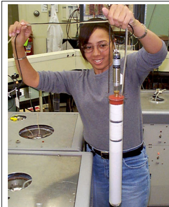
Initiating a freeze of a tin freezing point cell, as part of the calibration of an SPRT on the ITS-90.
