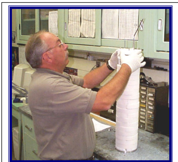
Fabrication of a center heater core for a new type of high-temperature furnace, used in the realization of the ITS-90.
