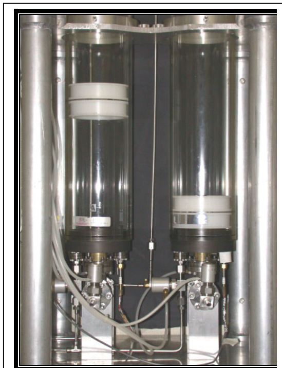
Figure 1. Close-up view of Hg-sealed pistons and prover tube assembly used for dry-gas mass determination in the NIST Gravimetric Hygrometer.
