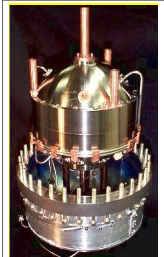
Figure 1. The 3 liter acoustic resonator, resting inside the lower part of a pressure vessel.
