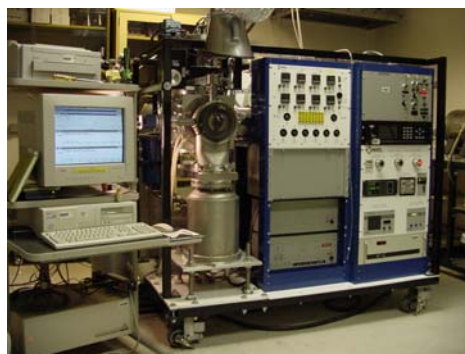
Bench scale laminar entrained flow (LEFR) reactor system and molecular beam mass spectrometer system.
