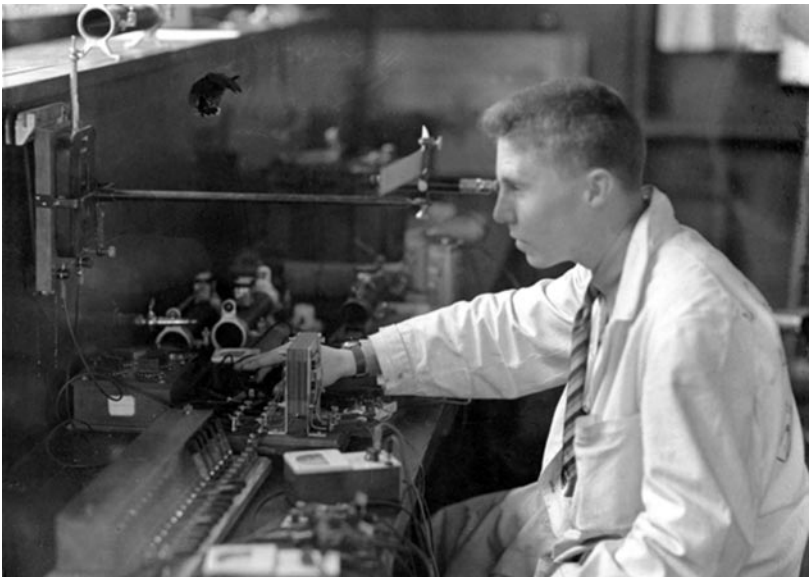
Figure 1 The author at the lab bench peering into the telescope of a ballistic galvanometer, taking data on magnetic hysteresis, 1943.
